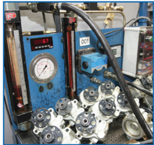
Remanufactured Power Steering Pumps Testing Station
